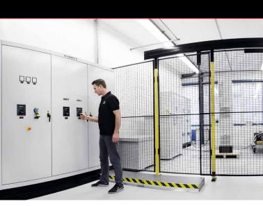
The Schaffner Drivelab is a tailored laboratory for testing and validation of Schaffner motor drive peripheral products such as EMI filters, harmonic filters, switching frequency filters and magnetic components. It offers our customers a certified and accredited laboratory infrastructure for the measurement of conducted emissions of electronic equipment according to international EMI regulations.
